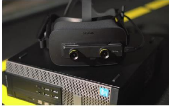
Fig. 15 Fused Reality® Flight system with ZED Mini Stereo Camera mounted on an Oculus Rift HMD.
