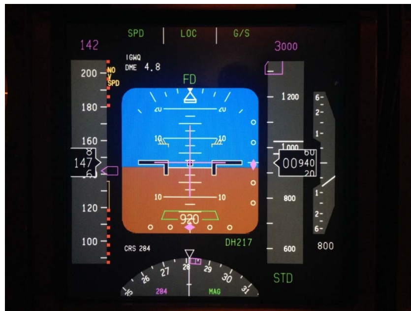
Figure 10: NASA Ames B747-400 simulator primary flight display with ILS flight director.
